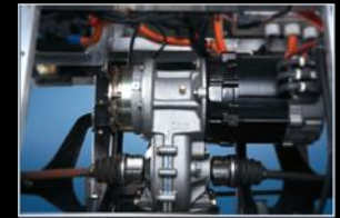
High Efficiency Motor and Gear reducer
